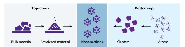
Figure 11. Basic schematic of the top-down versus a bottom-up approach to nanotechnology.
