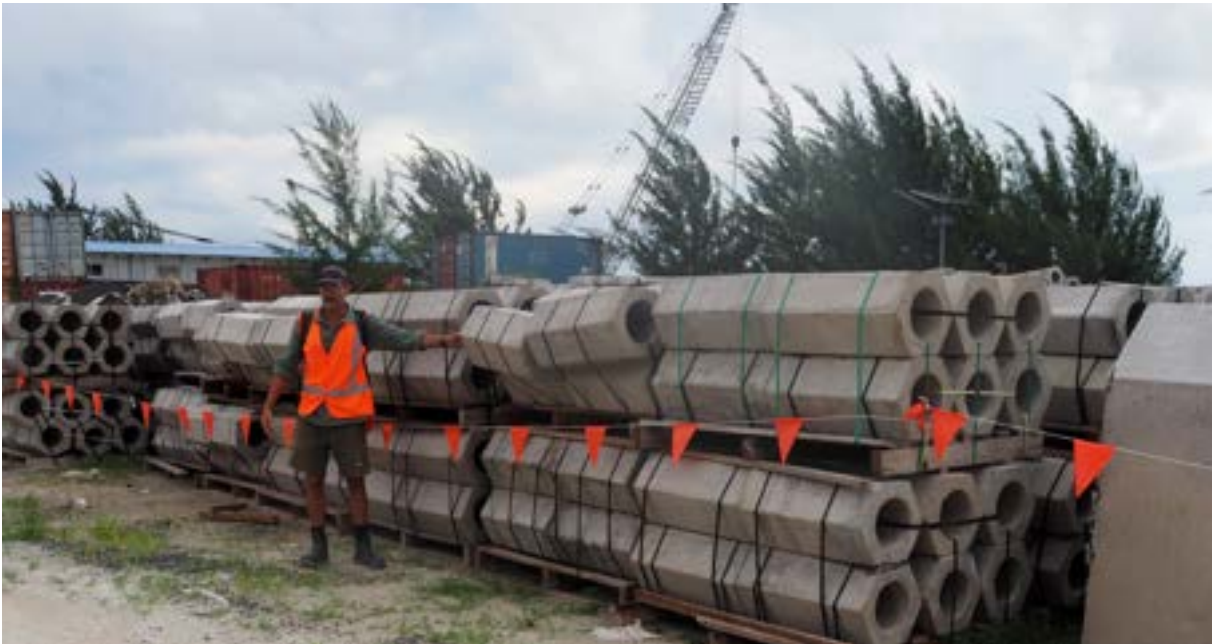
Concrete Seabees constructed in Fiji, destined for a coastal adaptation on Nanumea Island in Tuvalu.
